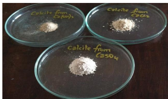
Figure 3: biocement produced for different calcium salts
