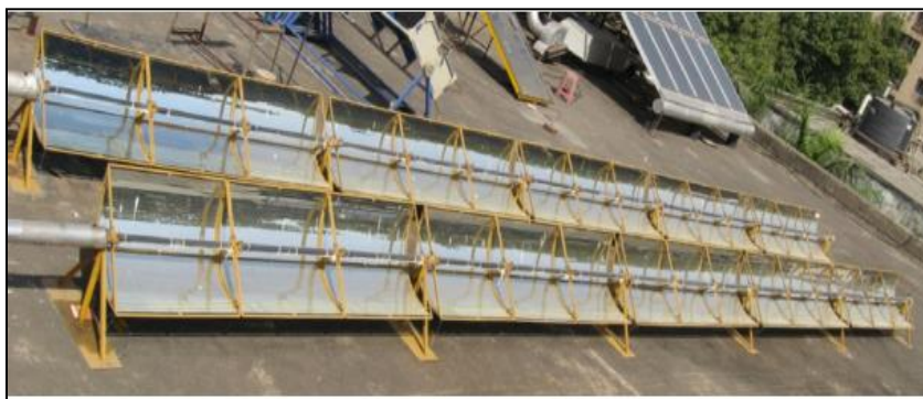
Fig 11: Compound Parabolic collector in India [20]
